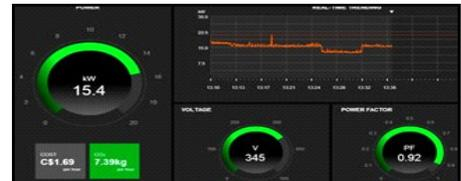
Real time monitoring and controls can spot problems in the BAS and plant operations based on energy usage not just performance. Usage spikes out of the norm indicate equipment or control malfunctions long before they would normally show up on the utility bill. Other issues concerning parts failure are also spotted in advance preventing costly emergency service.
