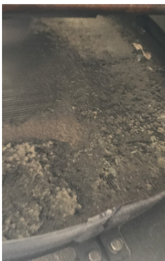
Radiator clogged causing overheating
